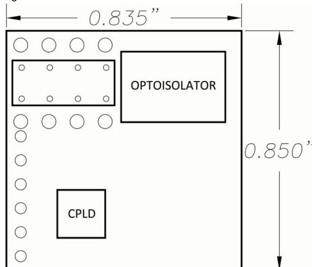
Once the jumpers have been located they may be set according to the diagram below. Please note that the four pins closest to the optoisolator are unconnected and can be used as jumper storage. It is recommended that needle nose pliers or tweezers be used to adjust the jumper settings. The power to the G213V must be turned off before any adjustment is to be made on the step pulse multiplier.
