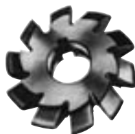
FIGURE 13—A 14-1/2° HSS involute gear cutter and a chart showing the cutting range of each size
