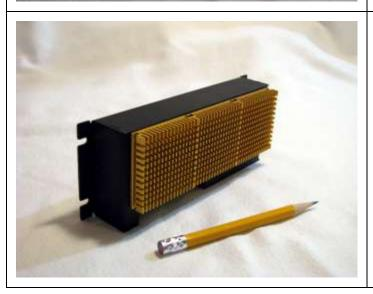
**Fifth**, peel of the second protective layer on the tape and stick down the heat-sink modules. After getting them in place press them down really hard to fully seat the tape.
