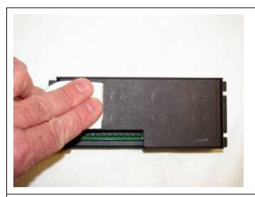
**First**, clean the back of your G540 with isopropyl alcohol and a small rag. Take care that no lint gets stuck to the ends of the screws.
