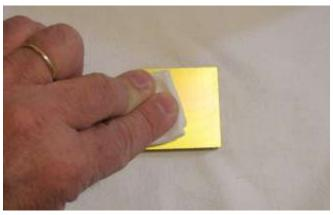
**Second**, clean the back of the heatsink modules with isopropyl alcohol as well.
