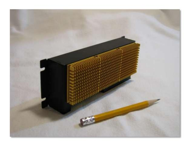
Thanks for purchasing the Soigeneris G540 Passive Heat-sink Kit. The kit contains three heat-sink modules and one strip of high performance heat-sink tape. You may notice that the tape is slightly smaller than the heat-sink modules, having a slight gap around the perimeter of the installed heat-sink actually increases the heat transfer.
