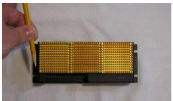
**Fourth**, don't peel off the second protective layer of tape yet. First do a test fit, get the heat-sink modules centered and make an alignment mark on one side.
