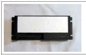
**Third**, peel the protective layer of one side of the tape and carefully apply as shown.
