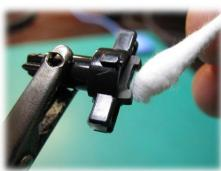
3) Insert key stem into matching aperture press lightly and take resistance reading.
